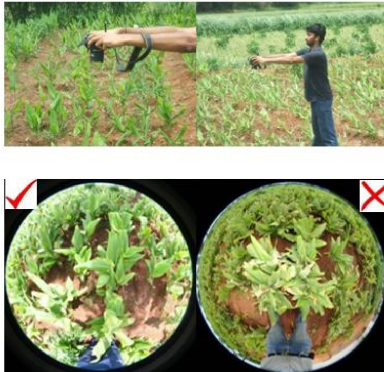
Figure 2-19: Example of taking Photograph Using Hemispherical Lens
